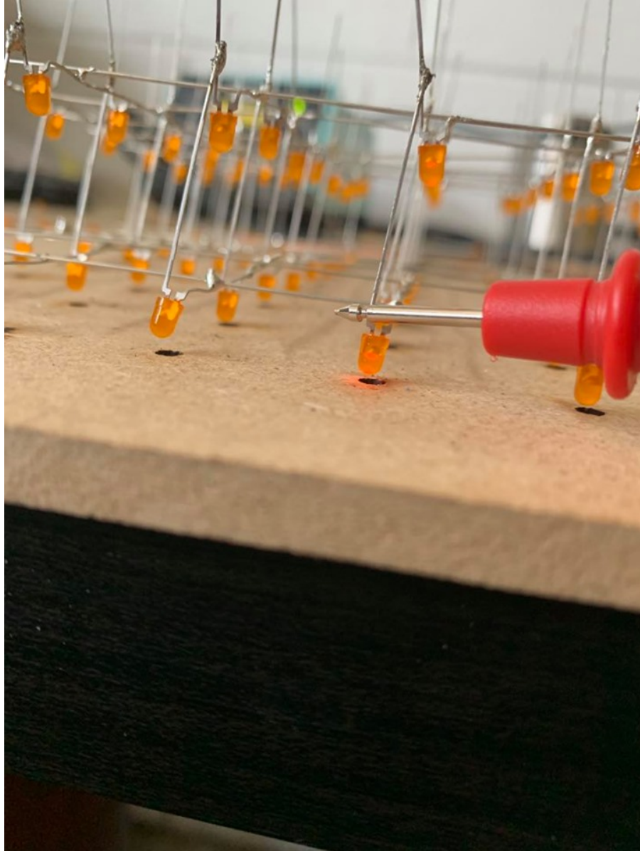
Figure 69: Testing of LED using Multimeter
